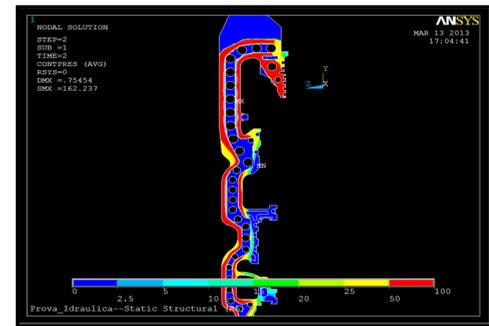
Contact pressure on the contact surface red indicates high pressure (50 - 100 MPa) blu indicate very low pressure (0 - 2.5 MPa).
