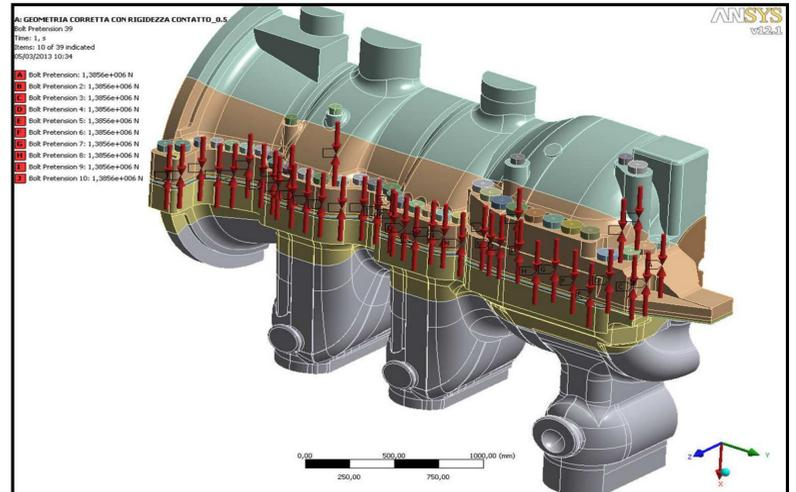
Preloads of the connecting bolts have been applied, as well as the internal water pressures, corresponding to the test pressure in the 3 different internal sections.
