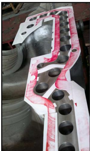
Photo of flange equipped with films after test: dark red indicates pressure equal or above 50 MPa white indicates pressure equal or below 10 MPa.
