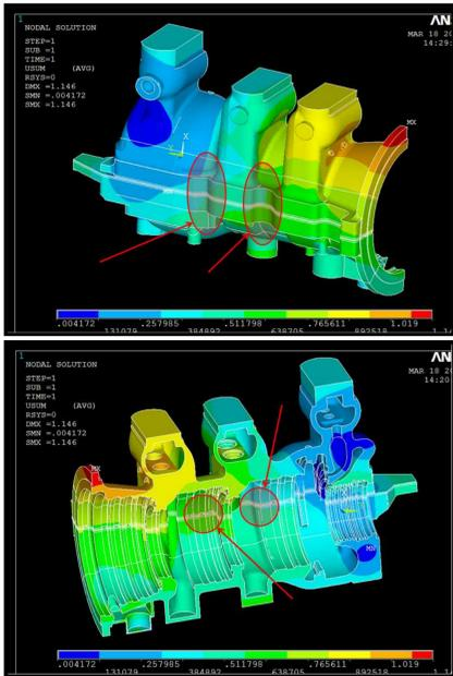
Model of the half casing showing points at the flange where leakage occurred during hydraulic test.
