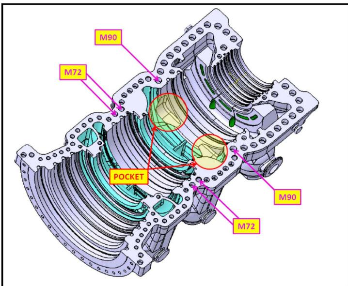
Sketch of the casing with indication of the suggested modifications: Size of some bolts has been increased (for increasing preloads) Two pockets (that have negligible influence on fluidynamic behaviour) have been introduced in the casing for increasing its local flexibility.
