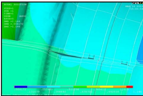
Gap between flange surfaces in one of the two critical points caused by the applied forces simulating the hydraulic test.
