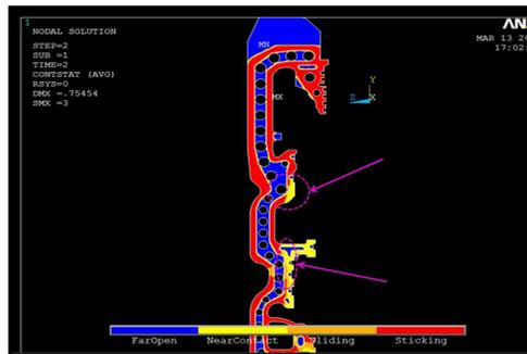
Contact status on the contact surface red is sticking contact, yellow is "near contact" arrows indicate leaking surfaces.
