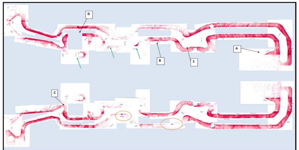
Scan of all films recombined after removal from flange. Green arrows indicate critical points in accordance with simulation where leakage could occur. D indicates a missing film. Other marks indicate parts where unexpected contact pressures were found, due to surface irregularities and insufficient load on bolts: in A pressure is below 10 MPa, in B pressure exceeds simulated values.
