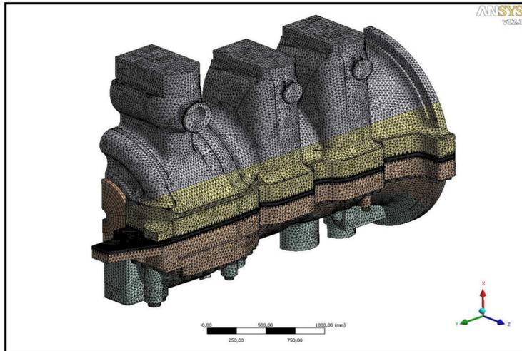
FEM model of the half casing. Symmetry about vertical plane and non-linear friction contact are used.
