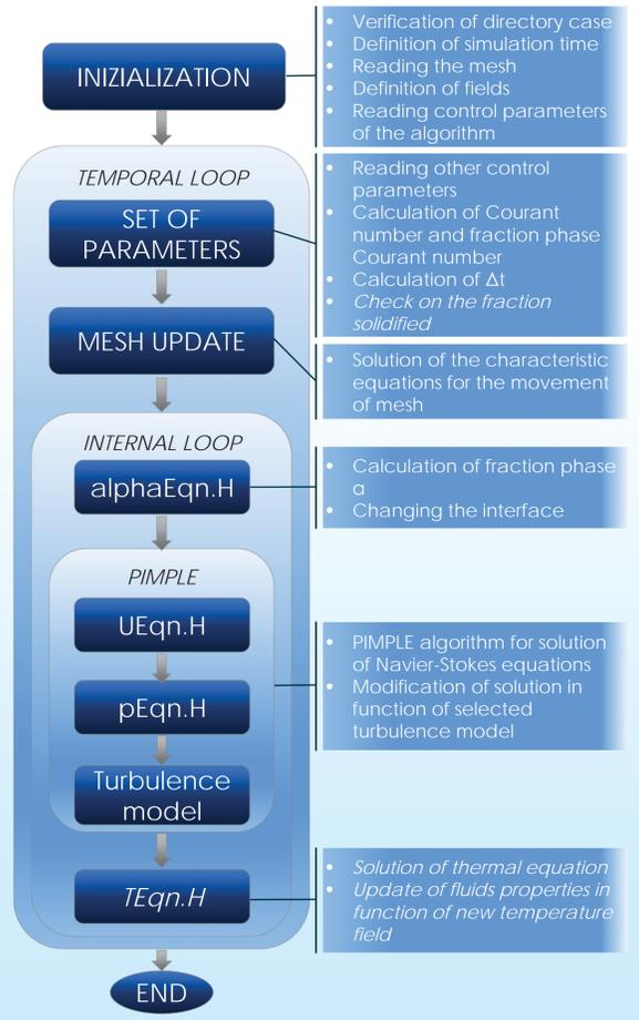
Algorithm for the numerical model implemented into a CFD code. Parts in italic font represent changes to the original solver.
