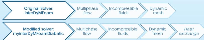
An existing solver, *interDyMfoam*, has been used as a basis for this project. The figure shows physical phenomena that are taken into account for the original solver and modified one. Heat exchange has been introduced adding two main features: computation of temperature field and temperature dependent fluid properties such as viscosity and density.
