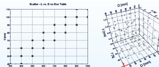
Two example graphs that show the distribution of experiments in the design space. The graph on the left gives the idea about the constraints imposed on the geometric variables. These designs have been written into an excel spreadsheet, reported below.
