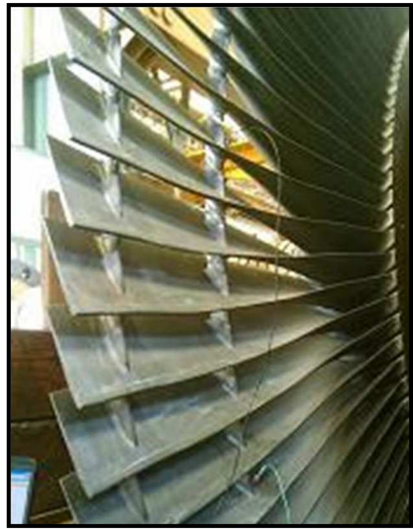
L-0 blade row: 120 blades with fir tree roots, grouped in packs of 8 blades by welded snubbers.
