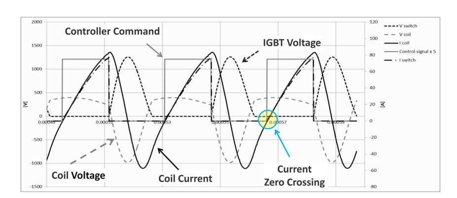
The multi physics circuital model simulation provides the power delivered to the inductor, voltage and current stresses on components and the frequency of the controller command.
