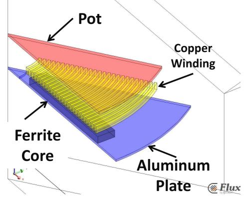
In 2D FEM, ferrite cores are replaced by a ferrite ring with an equivalent magnetic permeability. In 3D FEM, only a slice of the whole coil has been simulated. The simulations were performed with common pot materials like AISI409 and AISI430, nonlinear B(H) characteristic and resistivity about 0.6-0.7 [ $\mu\Omega$  m].
