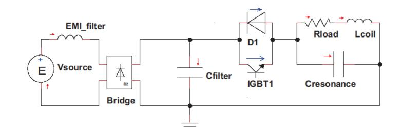
The **control variable is the T\_{on}**, while the Period  $(T_{on}+T_{off})$  depends of natural oscillation of RLC circuit. Moreover the coil current has not zero mean value.
