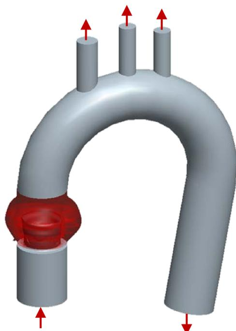
**Figure 2** – CAD 3D geometry of the flow domain within the aortic arch. The red zone represents the Valsalva Sinuses where the prosthetic valve is placed.
