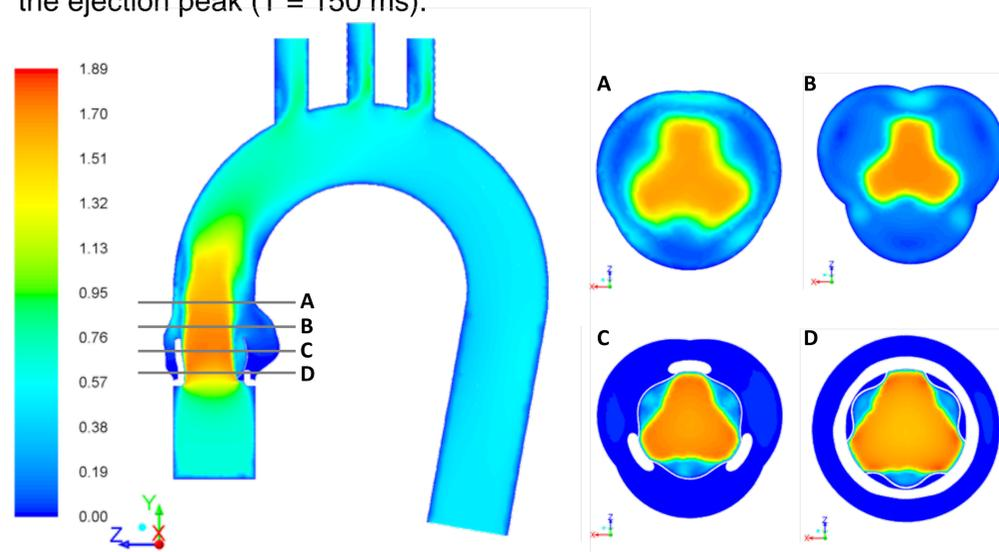
**Figure 3** – Contours of Velocity Magnitude [m/s] in the aortic arch and in four different locations within the Valsalva Sinuses.
