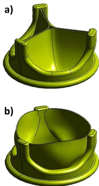
**Figure 1** – CAD images of the closed (top) and open (bottom) configurations of the optimized polymeric valve.
