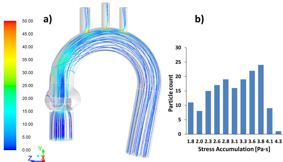
**Figure 4** – (a) Particle trajectories coloured by Scalar Stress [Pa]; (b) Frequency distribution of the Stress Accumulation [Pa·s] in the model.
